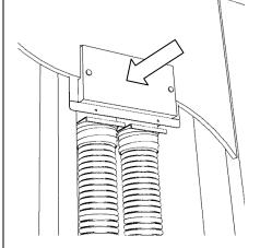
**7.** If only one duct is required for the installation, press the red plug into the unused connector.
