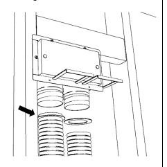
4. Insert ComfoTube with O-ring all the way into the plastic connector and press retaining clip fully into grooves.
