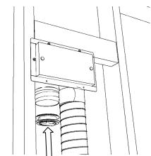
8. The red plug must not be left flush with the end of the black connector. This will allow air to leak through the slots in the connector.
