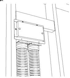
**6.** Cut drywall to fit around dust cover. Keep dust cover installed throughout construction!
