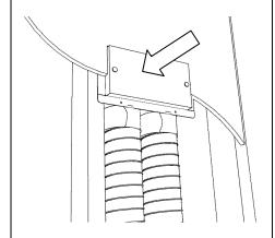
7. If only one duct is required for the installation, press the red plug into the unused connector.
