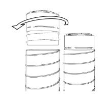
**3.** Seal end of ComfoFlex ducts to connector with UL 181B-FX tape. Cover slots in connectors with tape to avoid leaks.
