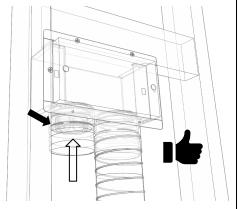
For ComfoTube (white plastic) ducts. See alternate instructions for ComfoFlex (gray fabric) ducts.
