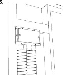
**6.** Cut drywall to fit around dust cover. Keep dust cover installed throughout construction!
