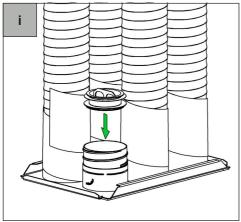
To cap an un-used port, install twist connector and push red plug all the way to the bottom past slots.
