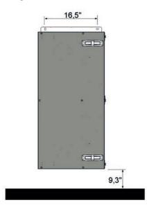
**Mount** the ComfoAir against a wall with a minimum mass of 0.28 lb/in² (200 kg/m²).
