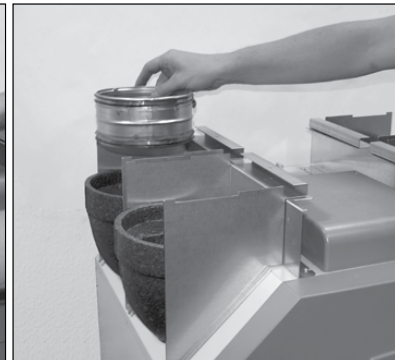
6. Insert the 160 mm nipple into the CA 350
