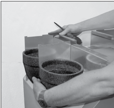
4. Attach the mounting to the U-profile
