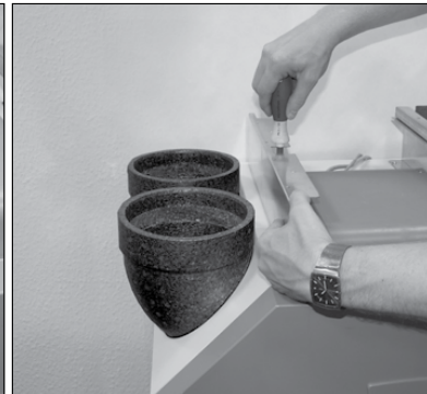
3. Locate U-profile and screw onto the CA 350
