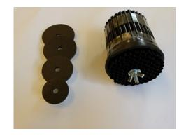
2. Insert ComfoSet with preinstalled reduction disk (dark foam side touching straws), washer and wingnut completely into air duct until soft foam seals tight.
