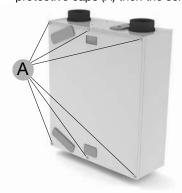
Remove the metal cover at the lower edge behind
